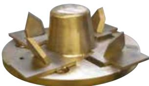
The Vortex reverse shredding Impeller : DIPCUT® is a conical Vortex impeller that becomes a "Shredder" when it changes direction of rotation. Coupled to smart automated command, this impeller changes automatically its direction of rotation when needed in order to cut snarled long fibrous materials and wipes, and then remove them.
